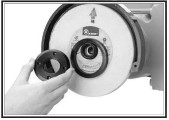
Figure 16. Exposing wheel spacer washer.
